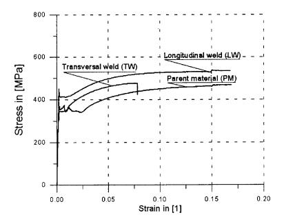
FIG. 6. Example of the stress-strain curves for three kinds of tensile specimens.
