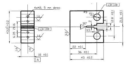
FIG. 4. Compact specimen used for CTOD and FCG tests.
