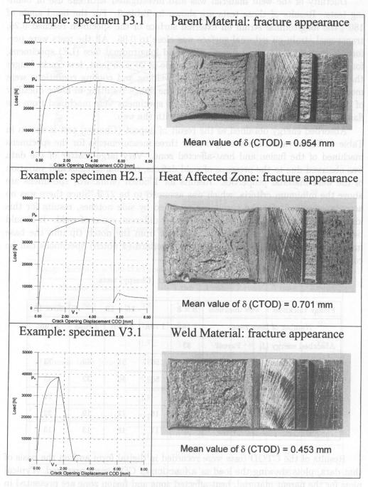
FIG. 7. Examples of load-COD plots and fracture appearance for PM, HAZ and FZ.
