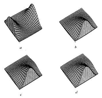
FIG. 2. The form of flexural vibrations of the panel depending on the number of approximation terms: 2a - one term (M = 1); 2b - two terms (M = 2); 2c - three terms (M = 3); 2d - four terms (M = 4).
