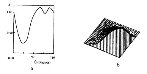
FIG. 3. Dependence of the frequency characteristic on angle  $\theta$ : 3a – first natural frequency  $(\lambda = \omega^2(\theta)/\omega^2(0))$  as a function of  $\theta$ ; 3b – the shape of vibrations surface z = 0 at  $\theta = 45^{\circ}$ .
