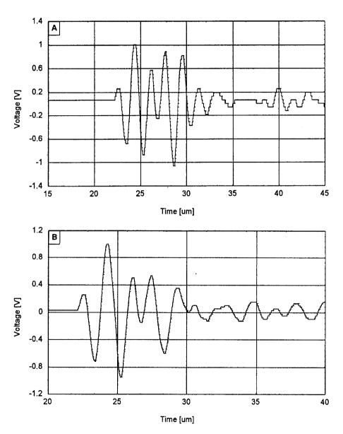
$\begin{tabular}{ll} Fig.~6. & Ultrasonic signals~from~two-different locations~of~water-saturated~s~ample~of~cancellous\\ & bone. \end{tabular}$
