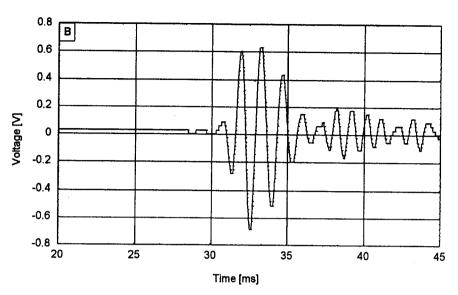
Fig. 2. Ultrasonics signals through the water-saturated samples of trabecular bone of thickness 8 (A) and 13 (B) mm.
