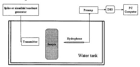
Fig. 1. Experimental setup for the ultrasonic immersion technique.
