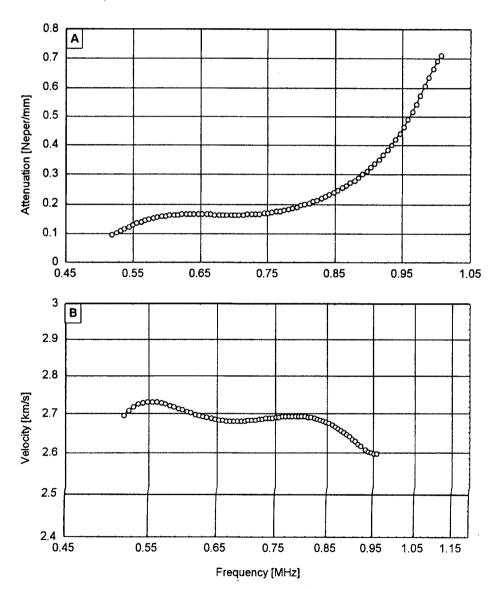
Fig. 5. Attenuation (A) and phase velocity (B) of the fast wave for water-saturated cancellous bone.
