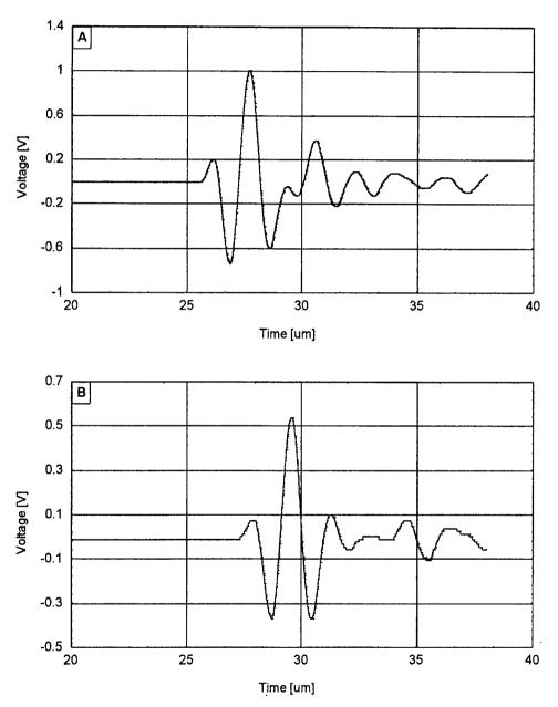
Fig. 3. Ultrasonics signals through the intact trabecular bone of thickness 8 (A) and 13 (B) mm
