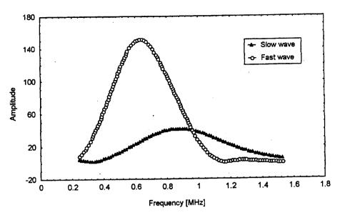
Fig. 4. Amplitude spectra for fast and slow ultrasonic pulse wave in water-saturated trabecular bone.
