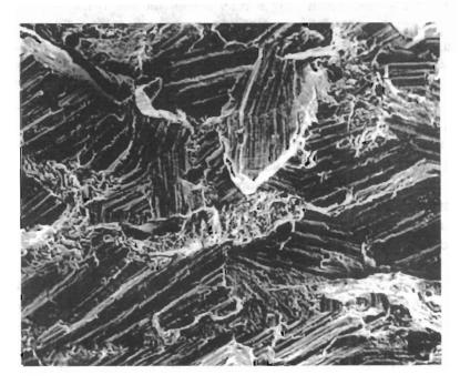
FIG. 4. Scanning electron micrograph of the tensile fracture surface for the longitudinal direction for a round tensile specimen artificially aged at 185 °C for 18 hours (170X).
