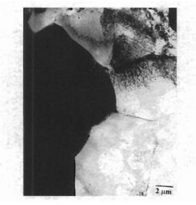
FIG. 2. Dark field TEM micrograph showing the microstructure of the Al-2.6wt.% Li-0.09wt.% Zr alloy in the overaged condition, artificially aged at 185 °C for 225 hours.
