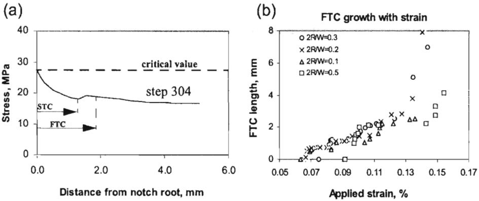
FIG. 12. (a) stress distribution at  $(1, y, 0.125)$  for  $2t = 1$  mm and  $2R/W = 0.5$ . (b) transverse damage growth with the influences of the notch sizes.
