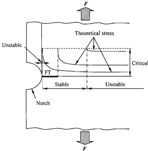
FIG. 13. Schematic representation of the transverse cracking mechanisms.
