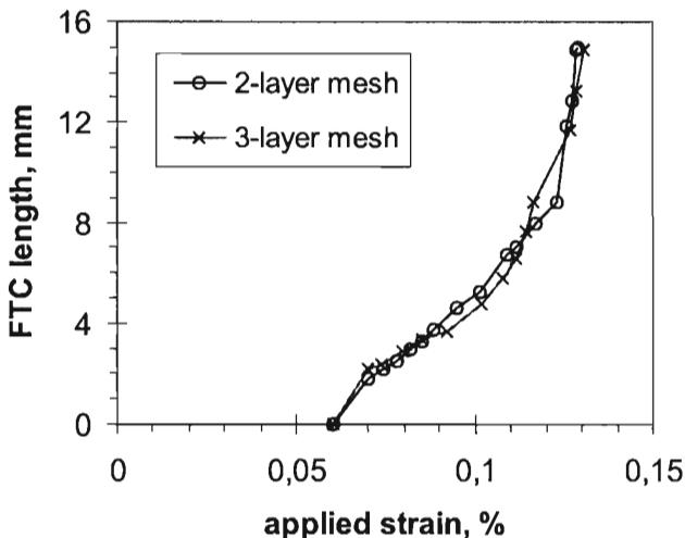
FIG. 5. The influence of the element number over the thickness of each lamina on the simulated FTC growth in a laminate with  $2t = 6$  mm and  $2R/W = 0.25$  ( $R = 5$  mm). Here 2/3-layer mesh means that the 0-layers and 90-layers are respectively modelled by using 2 elements or 3 elements in the thickness direction.
