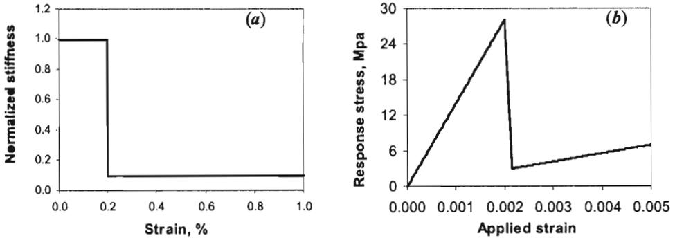
FIG. 2. (a) the normalized stiffness reduction of the 90° layers, (b) the local response of the 90° layers to the applied strain.
