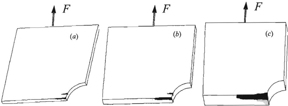
FIG. 9. Transverse cracking patterns at about the same applied strain,  $\epsilon_{app} = 0.11$  (a)  $2t = 1$  mm, (b)  $2t = 2$  mm and (c)  $2t = 6$  mm, views of the lower symmetric parts.
