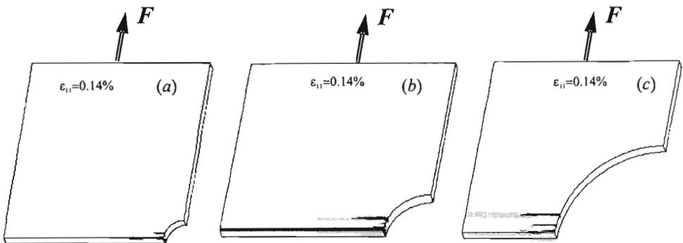
FIG. 11. Notch size effects on the multiplication of transverse cracks for  $2t = 1$  mm Laminate at  $\epsilon_{app} = 0.14\%$ : (a).  $2R/W = 0.1$ , (b).  $2R/W = 0.2$ , (c).  $2R/W = 0.5$ , views of the lower symmetric parts.
