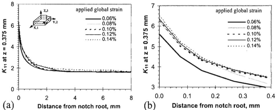
FIG. 8. (a). Stress concentration (at  $x = 0$ ) and redistribution at the mid-surface of the  $0^\circ$  ply as a function of transverse cracking,  $2t = 1$  mm and  $2R/W = 0.2$ . (b). Enlarged initial part of (a).
