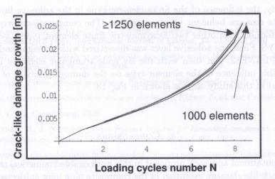
FIG. 12. Joint life sensitivity to the finite elements number in adhesive layer (vertical sensitivity).
