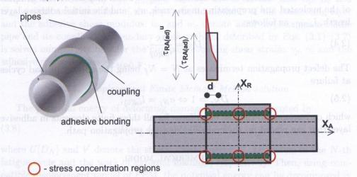
FIG. 1. Pipe-to-pipe adhesive connection: 3D and 2D views.
