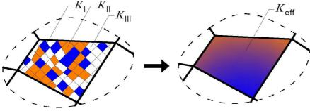
FIG. 2. Approach of local numerical homogenization.
