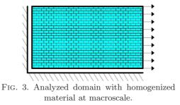
The load intensity q is equal to 1. Three random material distribution cases are presented in Fig. 4. The number of degrees of freedom is equal to 4290 in each case. Subsequently, the whole domain was discretized with one coarse element with eight degrees of freedom. Horizontal displacements along the righthand side edge for three distribution cases are shown in Fig. 5–7. Red solid line
