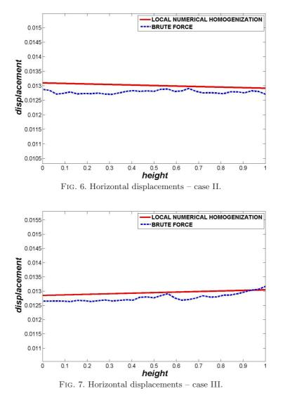
shows LNH solution, blue dashed curve shows the solution obtained using the fine mesh. Differences in solutions do not exceed 1 percent. Axis y limits in the graph are set to interval  $[0.9u_{\text{max}}, 1.2u_{\text{max}}]$ . Otherwise, the graphs of both solutions would be indistinguishable.
