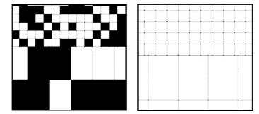
FIG. 10. Incompatibility of the fine meshes at the interface of layers.
