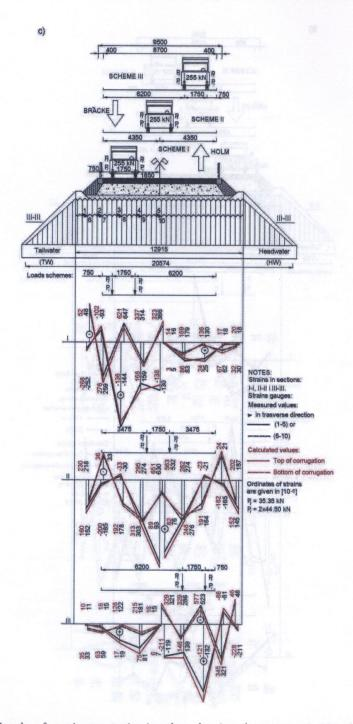
FIG. 9c. Graphs of maximum strains in selected points (gauges no. 1–20 in longitudinal direction) of steel shell structure in cross-sections of the span: c) III–III.
