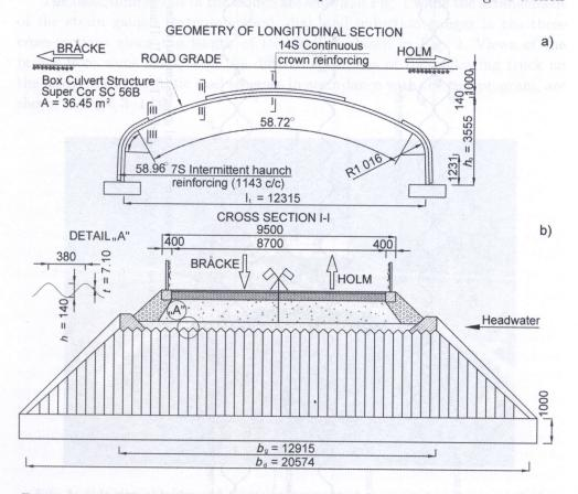
FIG. 1. Road bridge in Gimån, Sweden, made form Super Cor SC-56B corrugated plates: a) longitudinal section geometry and b) cross-section I–I.
