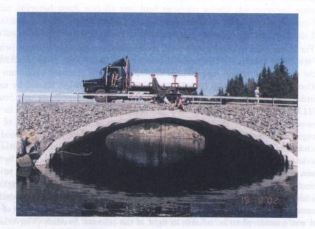
FIG. 3. Side view of bridge and *Scania* ballasting truck during tests (asymmetric load scheme I). Visible tripods for fixing displacement gauges.
