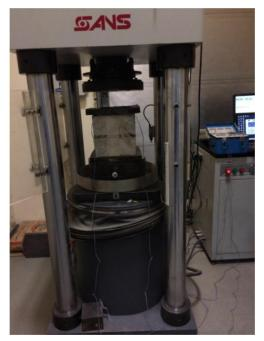
FIG. 3. Test setup consisting of compression machine, strain gauges and data logger.
