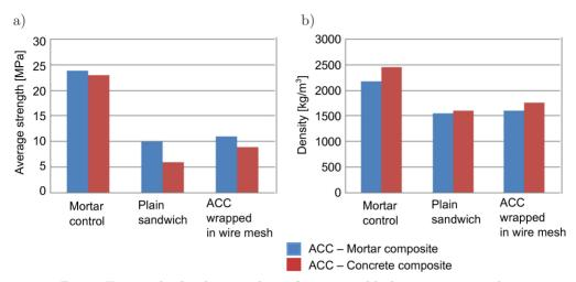
FIG. 5. Test results for the second set of composite block specimens at 3 days using a 3.0 MPa AAC: a) average strength, b) density.
