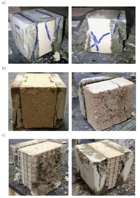
FIG. 6. Failure modes for AAC-sandwich specimens: a) plain, b) grooved, c) wire mesh.
