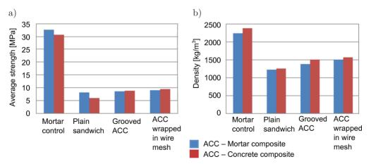
FIG. 4. Test results for the first set of composite block specimens at 7 days using a 1.8 MPa AAC: a) average strength, b) density.
