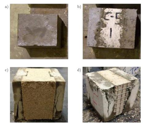
FIG. 2. A set of specimens used in the test program: a) control, b) plain sandwich, c) grooved sandwich, and d) wire mesh sandwich.
