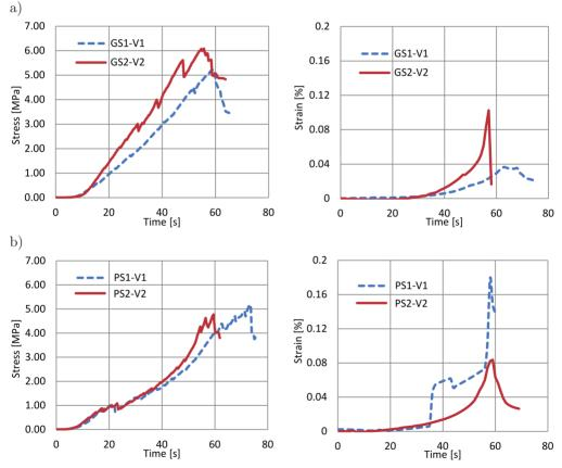
FIG. 10. Variation of stress and strains with time for grooved (a) and plain (b) sandwich composites at low and high quasi-static rates.
