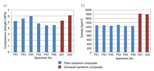
FIG. 9. Compressive strengths and corresponding densities of grooved and plain sandwiches at quasi-static loading rates: a) compressive strength, b) density.
