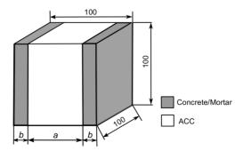
FIG. 1. 3D view of composite block.
