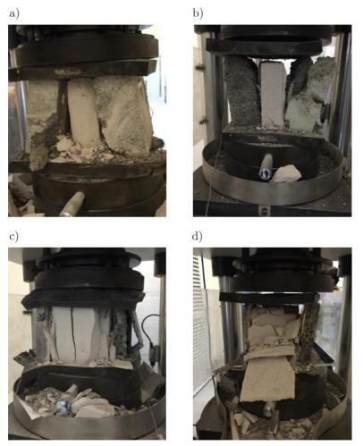
FIG. 11. Failure modes of plain and grooved sandwich specimens at different loading rates: a) GS1, b) GS2, c) PS1, d) PS2.
