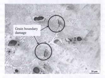
FIG. 6. Free-machining steel strained to 0.3 at 1273 K at  $\dot{\epsilon} = 0.01 \text{ s}^{-1}$ .
