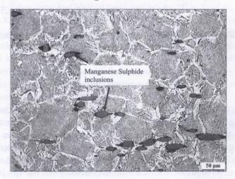
FIG. 3. Microstructure of free machining steel (after soaking) prior to deformation.
