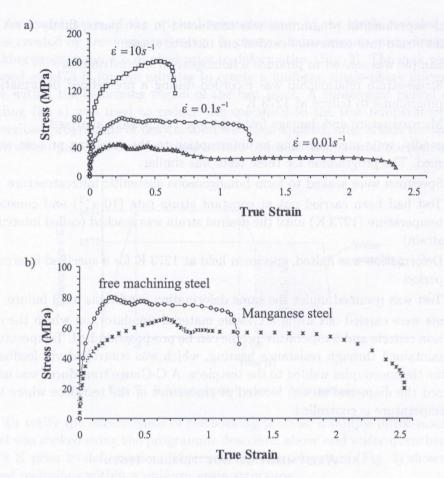
FIG. 4. Stress-Strain curves for a) free machining steel at 1273 K and b) free machining steel and CMn steel at 1273 K and  $\dot{\varepsilon} = 0.1 \text{ s}^{-1}$ .
