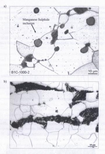
FIG. 1. Original microstructure of the test materials: a) Free machining steel and b) Manganese steel.
