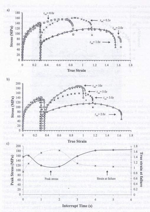
FIG. 8. Interrupted tests. a) Interruption time 0-2 s, b) interruption time 2-10 s, and c) summary of reloading properties.
