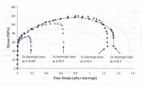
FIG. 7. Flow-stress on reloading after an interruption period.
