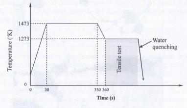
FIG. 2. Soaking applied prior to deformation.
