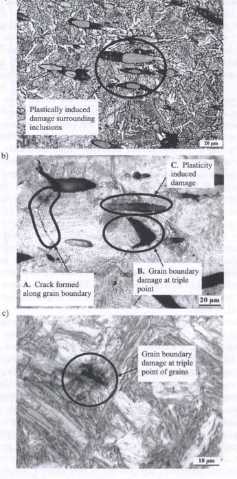
FIG. 5. Damage features of tested samples close to failure. a) free-machining steel at  $\dot{\varepsilon} = 10 \,\mathrm{s}^{-1}$ , b) free-machining at  $\dot{\varepsilon} = 0.01 \,\mathrm{s}^{-1}$ , and c) CMn steel at  $\dot{\varepsilon} = 0.01 \,\mathrm{s}^{-1}$ .
