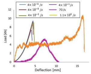
FIG. 13. Load-deflection curves at various deflection rates.
