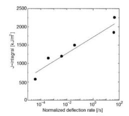
FIG. 7. Relationship between the J-integral and the normalized deflection rate of 3B test.
