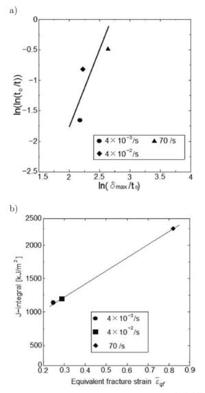
FIG. 15. a) The approximately linear relationship between  $\ln(\ln(t/t))$  and  $\ln(\delta_{\max}/t_0)$ , b) the relation between the Jintegral and equivalent fracture strain.
