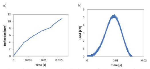
FIG. 11. The deflection-time curve (a) and load-time curve (b) obtained by SP test based on drop weight test method.
