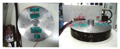
FIG. 6. The photograph of the load sensing block used in drop weight test.
