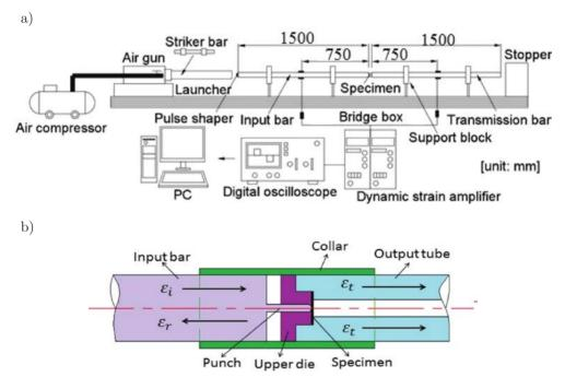
FIG. 12. The schematic picture of the established apparatus for the SP test based on SHPB method: a) whole of the apparatus; b) near the specimen including upper die and collar.
