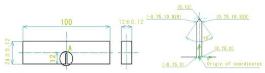
FIG. 2. The dimensions of the specimen for 3B test.
