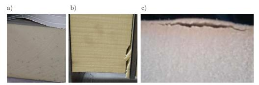
FIG. 1. Various types of delamination caused by: a) bending force, b) shear force, c) pressure.
