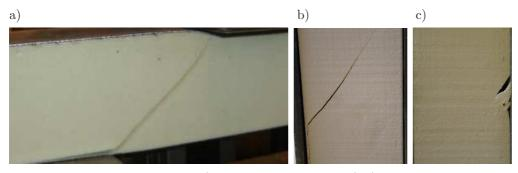
FIG. 2. Cracks obtained during: a) four point bending test, b), c) double lap shear test.
