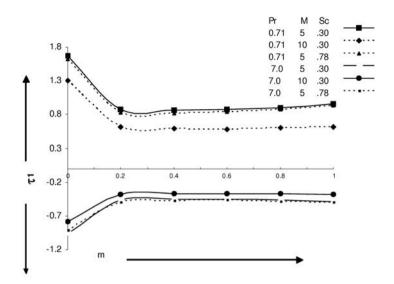
FIG. 8. Variation of shearing stress  $\tau_1$  for Gc = 2.0, G = -5.0,  $\Omega t = \pi/2$ .
