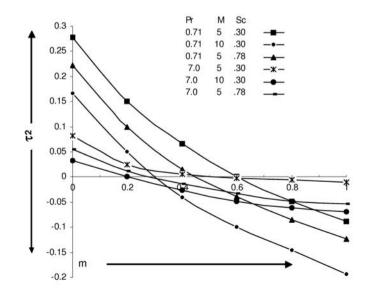
FIG. 9. Variation of shearing stress  $\tau_2$  for Gc = 2.0, G = 5.0,  $\Omega t = \pi/2$ .
