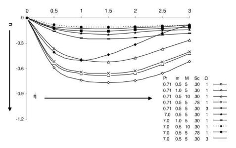
FIG. 1. Variation of velocity component u for Gc = 2.0, G = 5.0,  $\Omega t = \pi/2$ .
