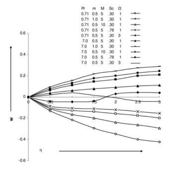
FIG. 4. Variation of velocity component w for Gc = 2.0, G = -5.0,  $\Omega t = \pi/2$ .
