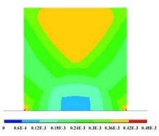
FIG. 15. Distribution of the material strength coefficient for square cell structure with orientation:  $\beta = 45$ .
