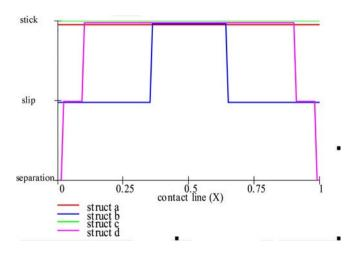
FIG. 6. Contact status (stick slip and separation zones) for different cell types.
