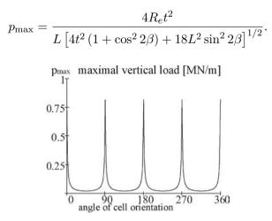
b) Honeycomb structure (isotropic material) analytical formulae:
