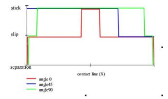
FIG. 9. Contact status (stick, slip, and separation zones) for different re-entrant cell orientation.
