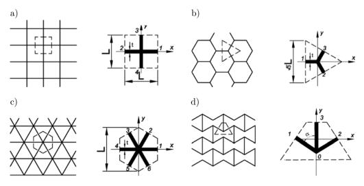
FIG. 1. Regular cellular plane structures, and their representative unit cells: a) square cell structure, square unit cell, b) 'honeycomb' structure, triangle unit cell, c) equilateral triangular structure, hexagonal unit cell, d) 'reentrant' structure, trapezoid unit cell.
