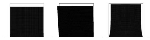
FIG. 10. Deformation of a square block made of reentrant cell microstructure for different cell orientations:  $\beta = 0$  deformation scale 3,  $\beta = 45$  deformation scale 2, and  $\beta = 90$  deformation scale 15.
