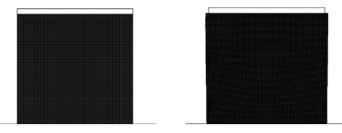
FIG. 14. Deformation of the body for different square cell orientations:  $\beta = 0$  deformation scale 10000,  $\beta = 45$  deformation scale 50.
