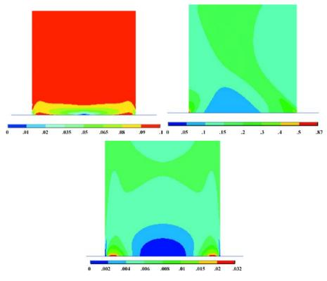
FIG. 11. Distribution of material strength coefficient for different reentrant microstructure orientation:  $\beta$ =0,  $\beta$ =45, and  $\beta$ =90.
