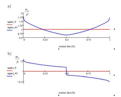
FIG. 12. Relative contact pressure and friction stresses distribution along the contact line for different square cell orientations.
