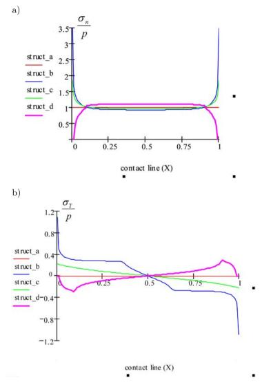
FIG. 5. Contact pressure and friction stress distribution along the contact line for different cell types.
