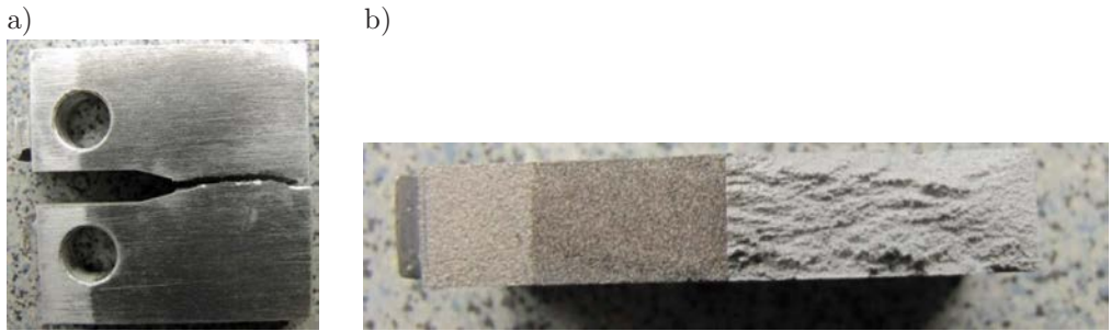
FIG. 11. Specimen made of the 44200+10% Saffil fibres composite after tests for K IC : a) specimen, b) entire fracture surface.
