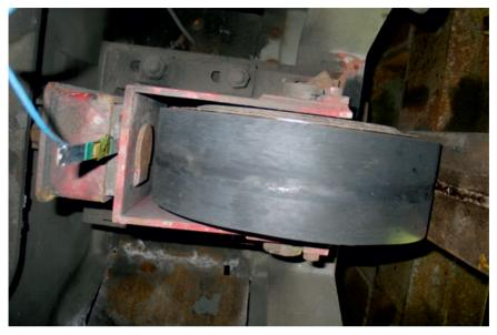
FIG. 18. Upper front guide with an attached strain gauge, general view.
