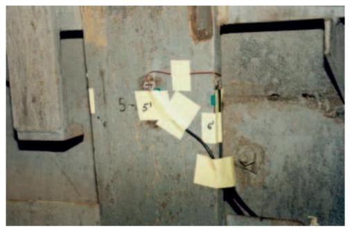
FIG. 24. Sensors TC5, TC5', TC6, TC6' fixed at the point where the mid-point string is connected with the hopper structure.
