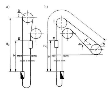
FIG. 1. Schematic diagram of a multiple rope hoisting installation: a) winder in the hoist tower; b) winder on the brink of the shaft.
