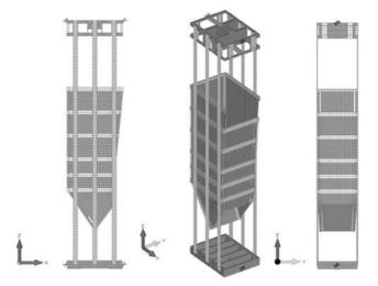
FIG. 3. Numerical (FEM) model of a skip of the lifting capacity 17 Mg.
