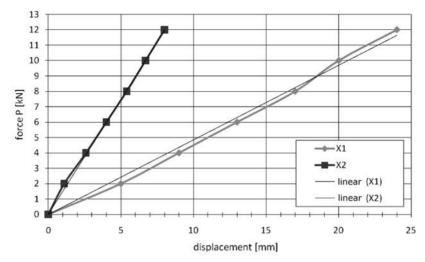
FIG. 16. Static characteristic of the lateral roller guide obtained by measurements  $(X_1 - \text{total displacement}; X_2 - \text{displacement of the roller housing})$  and its linearized form.
