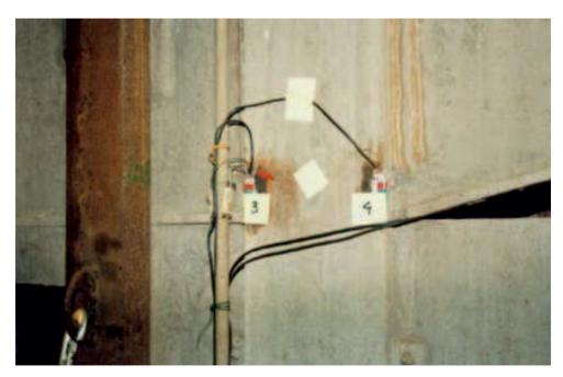
FIG. 23. Strain gauges TC3 and TC4 fixed to the mid-point string, at the attachment point to the head structure.
