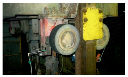
FIG. 6. Bottom guide bar assembly and attachment of tail ropes.
