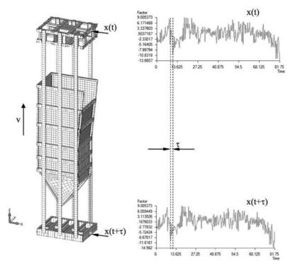
FIG. 8. Schematic diagram of skip loading by the displacement x(t).
