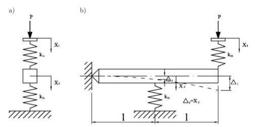
FIG. 14. Diagrams of the roller guide systems: a) front; b) lateral.
