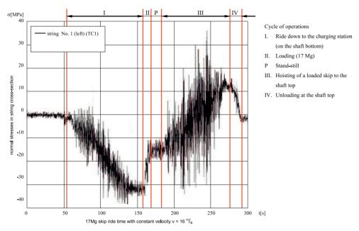
FIG. 26. Stress in the string cross-section registered by the sensor TC1.
