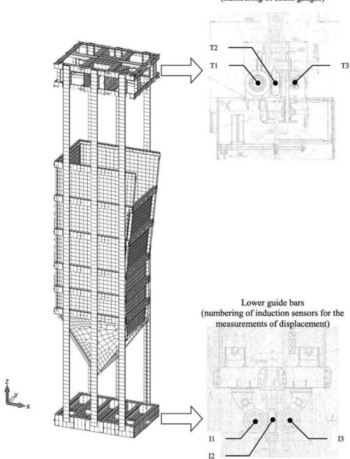
Upper guide bars (numbering of strain gauges)
