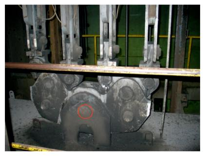
FIG. 5. Attachment of tail ropes for the skip with the support point in the FEM model revealed (red ring).
