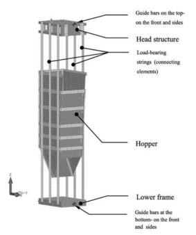
FIG. 4. Structural elements of the skip considered in the FEM model.
