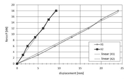
FIG. 15. Static characteristic of the front roller guide obtained by measurements  $(X_1 - \text{total displacement}; X_2 - \text{displacement of the roller housing})$  and its linearized form.
