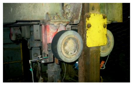
FIG. 19. Lower roller guide assembly with the attached induction sensors.
