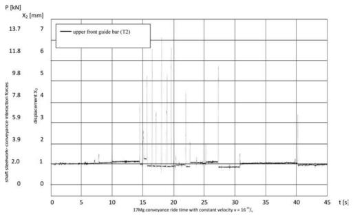
FIG. 20. Registered displacement  $X_2$  of the upper front guide bar (Travel I) during the ride up of a loaded conveyance.
