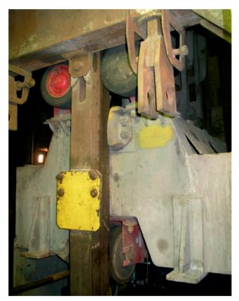
FIG. 7. Top guide bar assembly for the skip.
