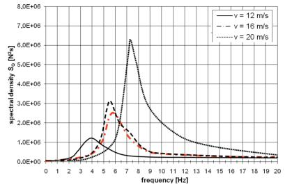
FIG. 21. Spectral densities of "shaft steelwork-conveyance interaction" forces obtained by solving of the 3D FEM model and experimentally (red colour).
