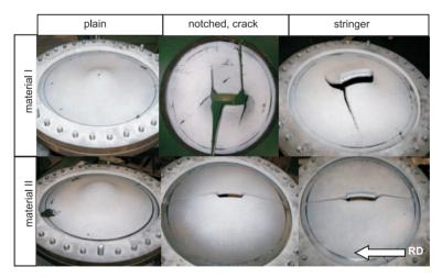
Fig. 6. Failure characteristics for two different materials at different pre-treatment states after biaxial testing.
