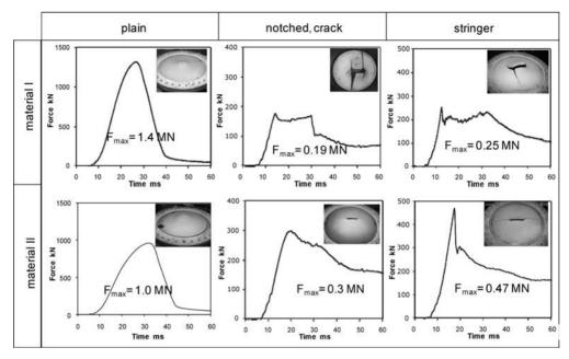
Fig. 7. Force-time behavior of two different materials with different stress-states at dynamic biaxial loading.
