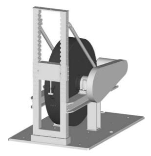
FIG. 8. Rotating wheel device of Nordmetall GmbH with a high amount of stored energy, by a 10 t flywheel (Ø2 m) for dynamic component testing of engineering materials.
