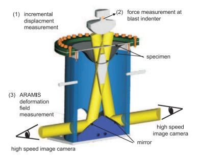
Fig. 5. Experimental test setup for high speed biaxial tensile-tensile-tests of steel plates, including high speed deformation field measuring system.
