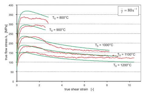
Fig. 4. Flow stress evolution of a low alloyed steel at high strains, high shear rate and high temperatures: comparison of experimental data and modeled data using the Hensel-Spittel approach [5].
