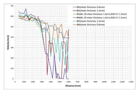
FIG. 14. Distance-velocity data using 40 mm rifled gun.
