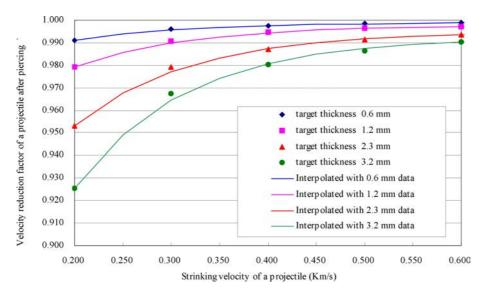
FIG. 1. Velocity reduction factors of projectile after piercing the metal plate.
