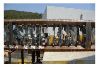
FIG. 10. Deformed plates, mid section.
