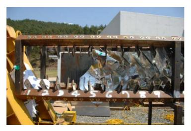
FIG. 9. Deformed plates, front section.
