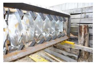
FIG. 11. Deformed plates end section.
