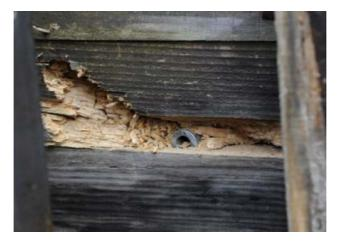
FIG. 12. Projectile wedged in wooden block.
