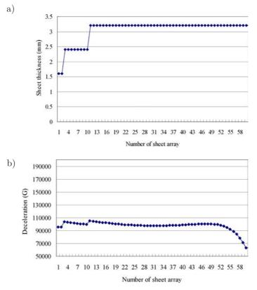
FIG. 2. Estimation of thickness distribution of plate array for soft recovery of projectile: a) thickness distribution of sheet array, b) estimated deceleration of a projectile.
