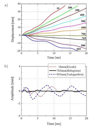
FIG. 14. Impact responses of *Tachi* with *koshirae*: a) variation of displacement with time at each location, b) oscillation of displacement.
