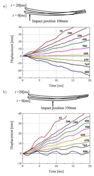
FIG. 8. Variation of displacement with time at each location: a) impact position of 100 mm from *Kissaki*, b) impact position of 350 mm from *Kissaki*.
