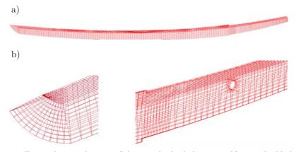
FIG. 11. Finite element division of the sword: a) whole region, b) near the blade tip and *Mekugi-ana* in the tang.
