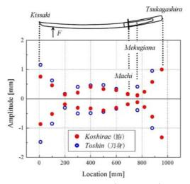
FIG. 15. Comparison of amplitudes for Toshin (tachi blade) and Tachi with koshirae.
