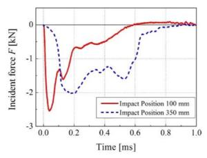
FIG. 7. Incident forces into Tachi blade.
